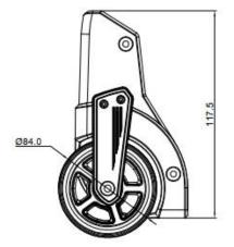
Item #: WR031 + WHL023 Material: ABS (Wheel housing) PP (Wheel Hub) TPU (Wheel Tire) Wheel diameter: 84mm
