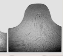
It causes the individual crystal grains to become elongated and flow in the direction of the deformation.
